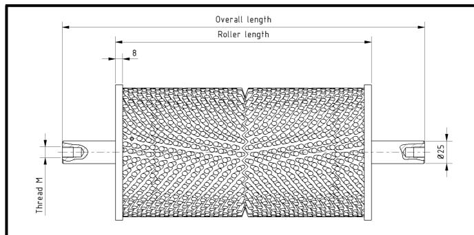
The **Brush Style spreader: BSW-ZZ** has a total diameter of 143 mm.
